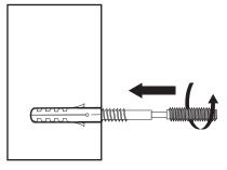
3. Screw a fixing bolt into each fixing plug using a 8mm spanner until the spanner contacts the wall.
