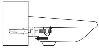
5. Screw a metal nut onto each fixing bolt to secure the basin. **Caution:** Do not over-tighten, as this may damage the ceramic.
