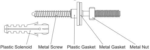
**NOTE:** These fixings are suitable for solid walls only. Plasterboard or stud walls may require specialist fixings (not supplied). **CAUTION:** Care should be taken when drilling walls and floors to avoid any concealed wires or pipes.
