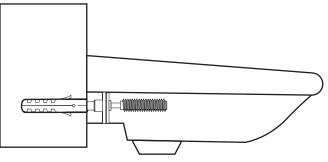
4. Place the basin in position against the wall. Locating the fixing bolts through the holes in the rear of the basin. Push a plastic washer followed by a metal washer, onto each fixing bolt.
